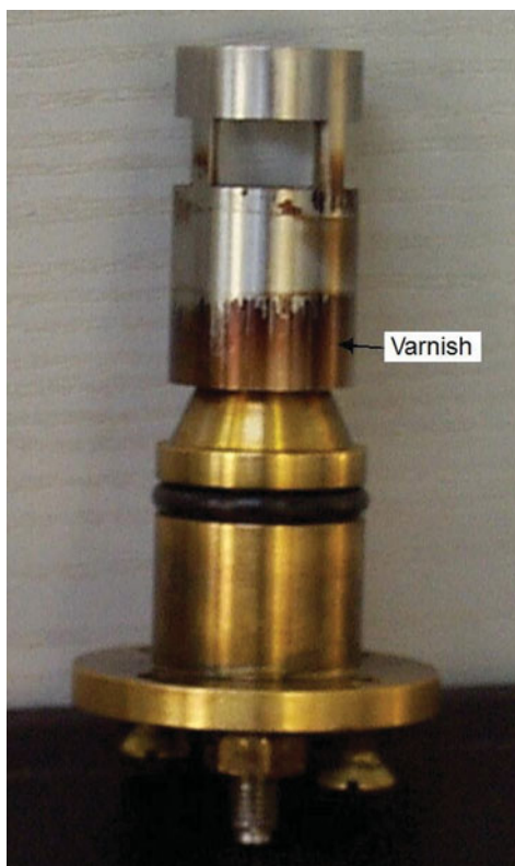
Fig. 1—Varnish on a valve piston (color figure available online). (Courtesy of Fortum UK.)
